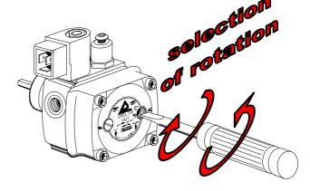
With the new Delta VU1 Universal pump it is now possible to substitute the pumps with shaft rotation clockwise and counter-clockwise, with delivery port on the right or on the left and one or two pipes system with only one unit, without difficulty and without special tools, the new pressure regulation gives a large pressure range without the necessity to change the spring.
