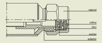
The disc atomizer 32 is the most flexible industrial nozzle for an output range of 460 kg/h up to 2200 kg/h.
